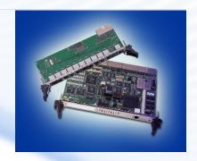
The IPnexus<sup>TM</sup> CPC5400 is an embedded Ethernet switch compatible with both standard CompactPCI® and PICMG® 2.16 backplanes. It is designed to be used as a high-speed interconnect within server blade chassis or as a core switch in fault-tolerant clusters of embedded systems.
