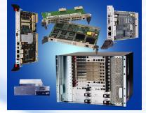
With the advent of packet-switched backplanes and intelligent shelf management, the basic definition of a standards-based platform begins to change. As platforms evolve to include these new and critical functions, they include not only the chassis, midplane, power and cooling architecture, but also the PICMG® 2.16 packet-switched backplane and PICMG 2.9 intelligent platform management interface (IPMI) standards.
